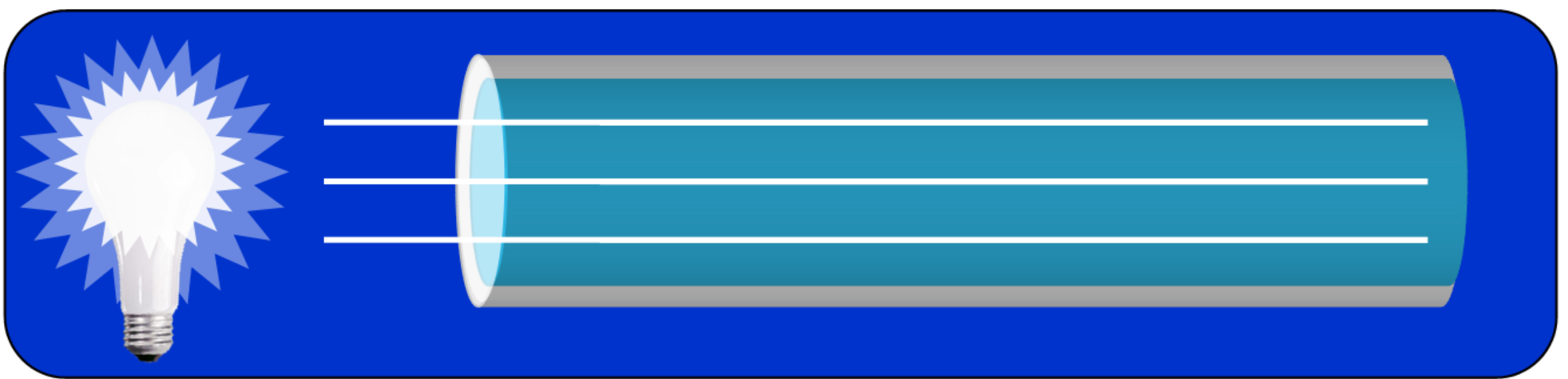
Single-mode fiber - Light enters at a single angle. Made for long distances.
