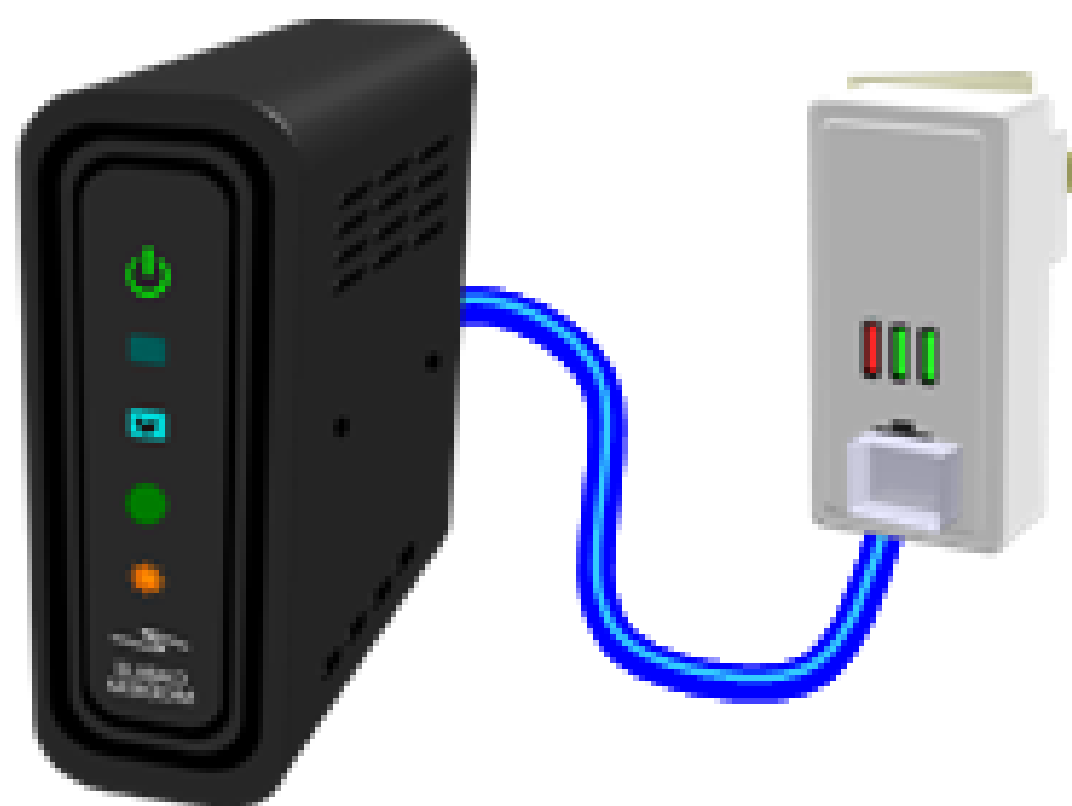
Modem plugged into a powerline network adapter.
