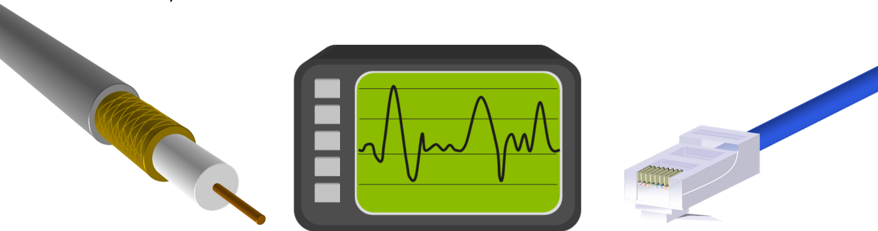
A TDR tests cables, such as coaxial and UTP.
