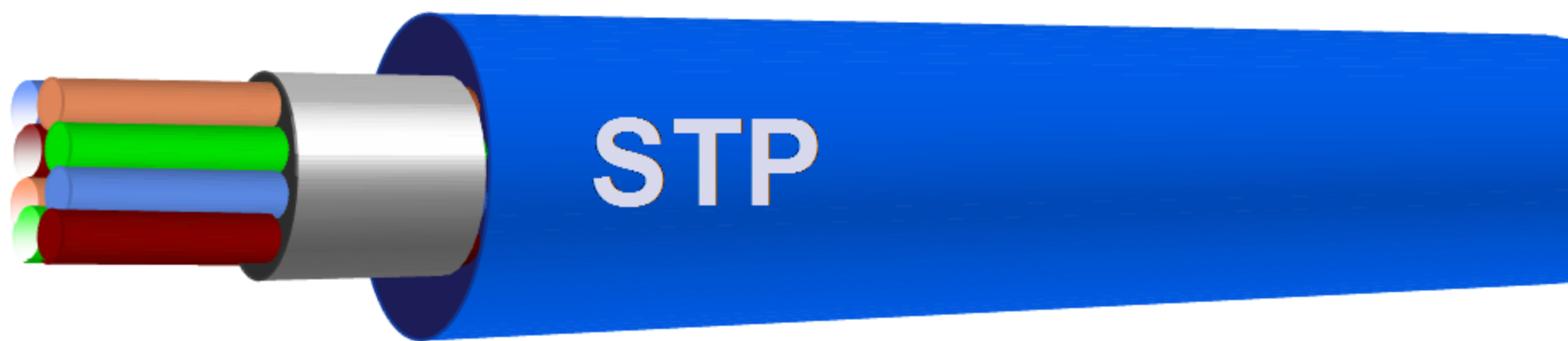
Shielded twisted pair (STP) cable adds a foil shield that covers the wires.
